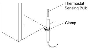
Figure 5 - Attaching Thermostat Sensing Bulb
